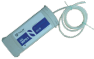
B. Modified cartridge (x 8) (pre connected to ink reservoirs)
