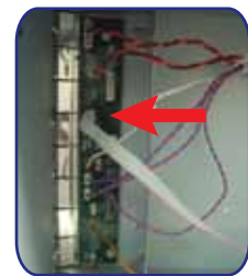
1f. Unplug the white ribbon cable from the PRINT MECH board connector marked "ISS P8".
