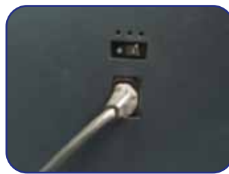
1b. Unplug the power cable from the back of the printer.
