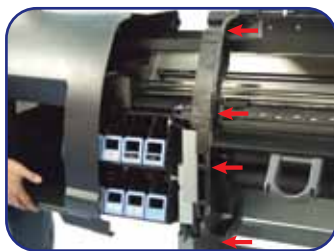
1d. Remove the left hand cover by removing the screws marked in fig.
