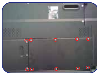
1e. Open the cover from the back of the printer (10 screws) This will enable access to the PRINT MECH board.
